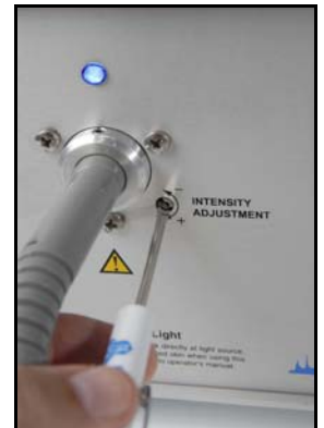
Intensity adjustment, with knob removed, performed with adjustment tool
