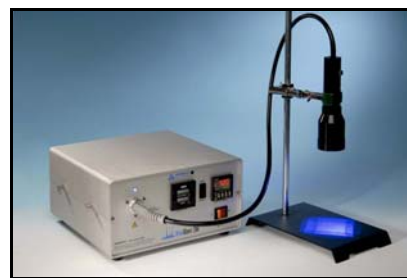
Rod Lenses Shown: BlueWave 200 with 8 mm rod lens (rod lenses require an 8 mm lightguide) 2" x 2" Area (~100 mW/cm 2 ) PN 38699 5" x 5" Area (~30 mW/cm 2 ) PN 38698
